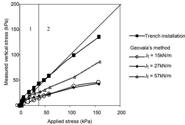
**Figure 4- Vertical stress over the pipe during construction (1) and surcharging (2).**
