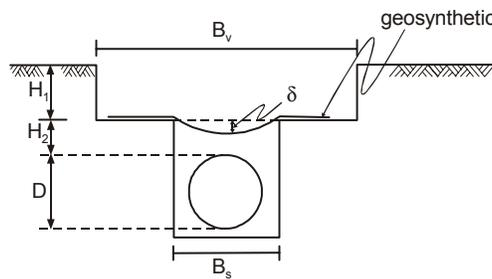
**Figure 1. Trench installation according to Geovala method.**
