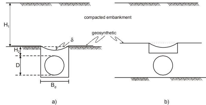
**Figure 2. Projecting pipe installation using the Geovala method: a) negative projecting pipe; b) positive projecting pipe.**
