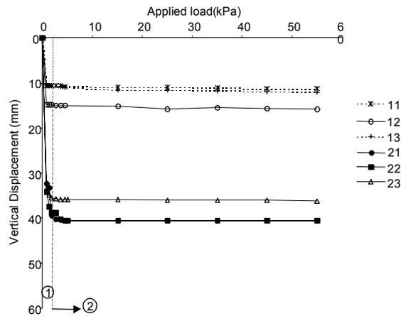
**Figure 3. Vertical displacement of geosynthetic bridging the trapdoor opening during construction and surcharging.**
