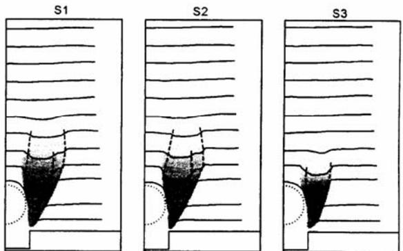
Figure 6. Failure mechanisms of the transverse sections of Model 4 (rigid pipe in dense backfill)
