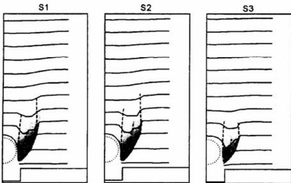
Figure 4. Failure mechanisms of the transverse sections of Model 2 (flexible pipe in dense backfill)
