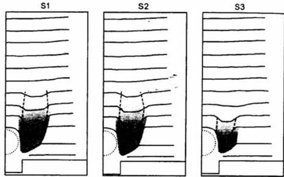
Figure 5. Failure mechanisms of the transverse sections of Model 3 (rigid pipe in loose backfill)
