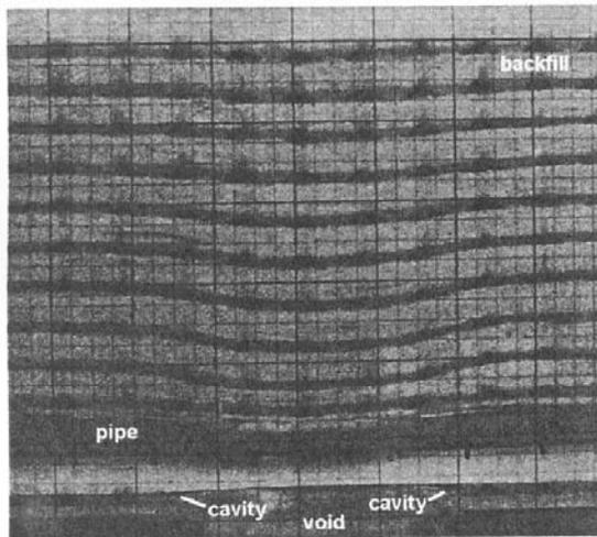
Figure 7. Failure pattern in longitudinal section of model 1 (flexible pipe in loose backfill)
