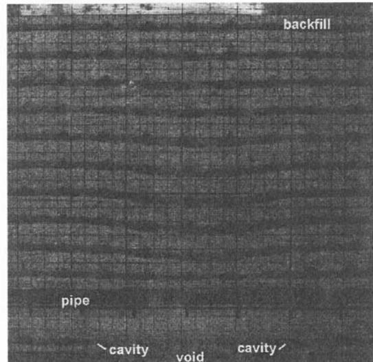
Figure 8. Failure pattern of longitudinal section of model 2 (flexible pipe in dense backfill)
