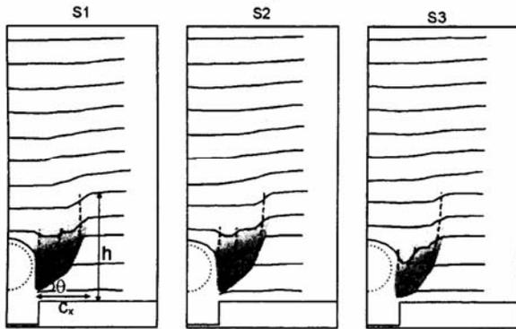
Figure 3. Failure mechanisms of the transverse sections of Model 1 (flexible pipe in loose backfill)
