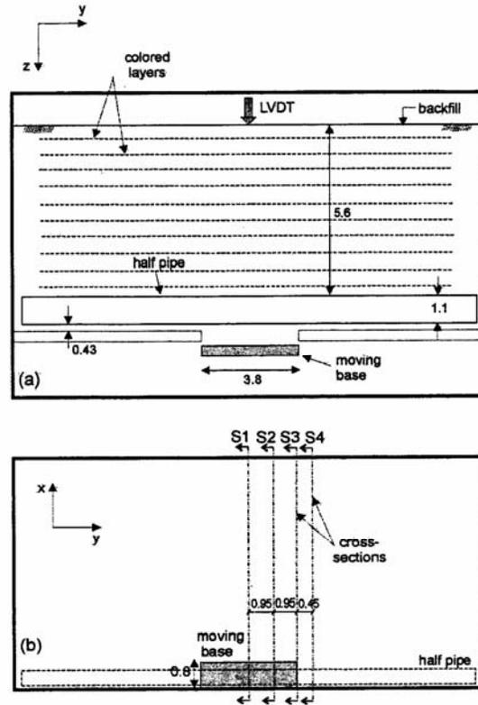
Figure 1. a) Scheme of model configuration; b) plan view of model showing positions of the transverse sections. Prototype dimensions (m)
