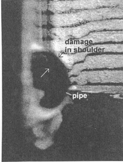
Figure 9. Damage experienced by the flexible pipe in the loose backfill (Section 1)
