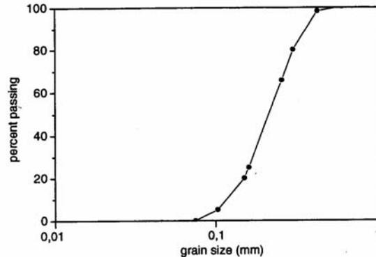
Figure 2. Grain size distribution of the sand used as backfill
