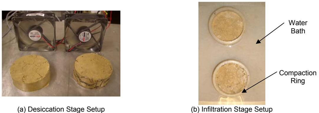
Figure 2. Testing Setup for the (a) Desiccation and (b) Infiltration Stages.
