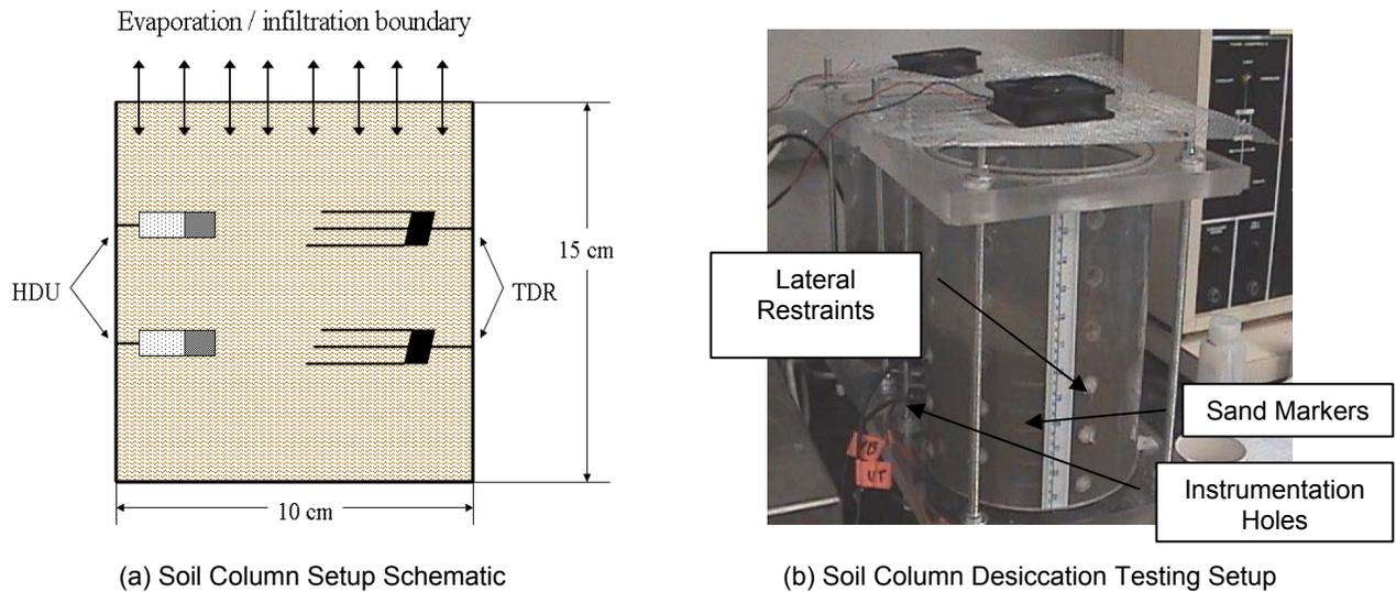
Figure 1. Soil Column Testing Setup (a) Schematic and (b) Desiccation Testing Setup.
