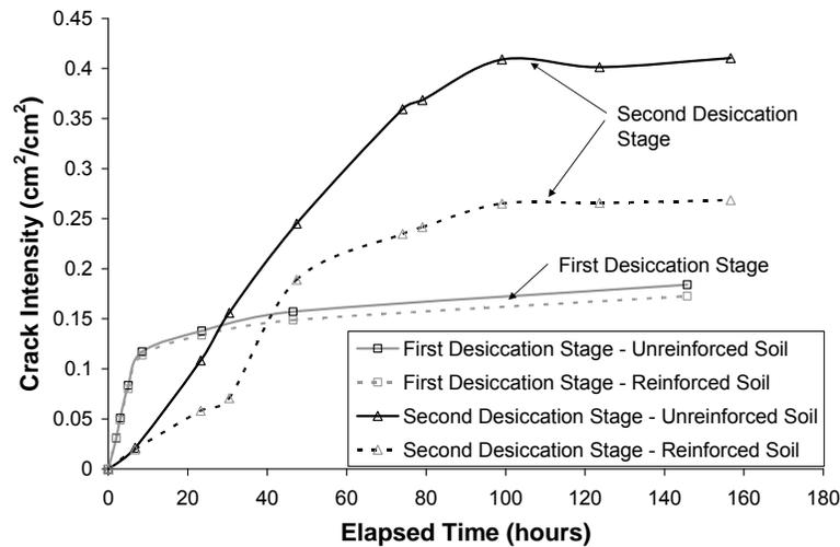
Figure 7. The Development of the Crack Intensity Factor (Including Sidewall Separation) With Time for the Second Desiccation Stage.
