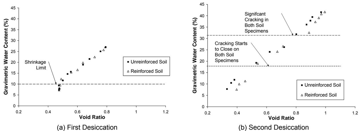
Figure 3. S-Curves for the Fiber-Reinforced and Unreinforced Eagle Ford Clay Specimens during the (a) First and (b) Second Desiccation Stages.
