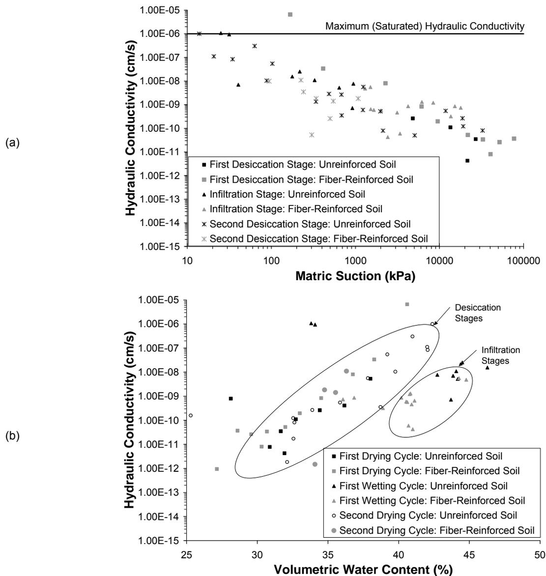
Figure 10. Change in Hydraulic Conductivity with Matric Suction (a) and Volumetric Water Content (b) for the First Desiccation Stage, Infiltration Stage, and Second Desiccation Stage.
