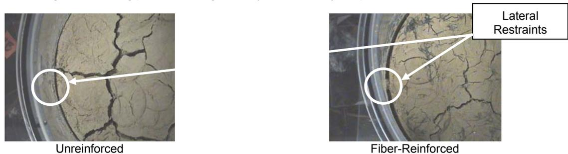
Figure 4. Radial Separation of the Soil Columns During the First Desiccation Stage.
