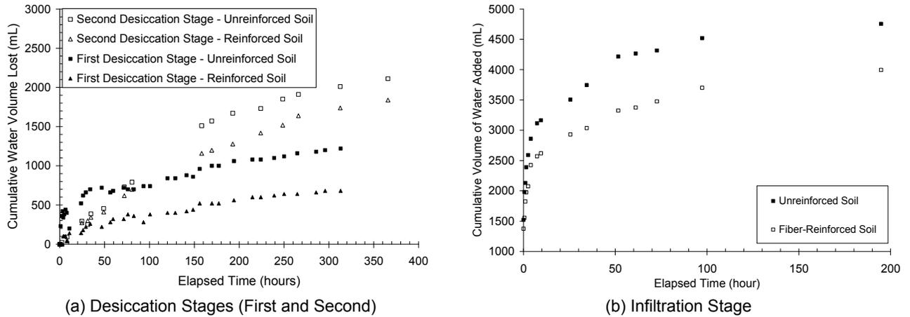
Figure 8. Change in Volume of Water with Time for the (a) Desiccation Stages and (b) the Infiltration Stage
