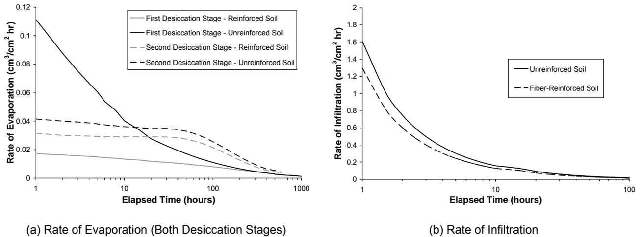
Figure 9. Change in the Rate of Evaporation (a) and Infiltration (b) with Time.
