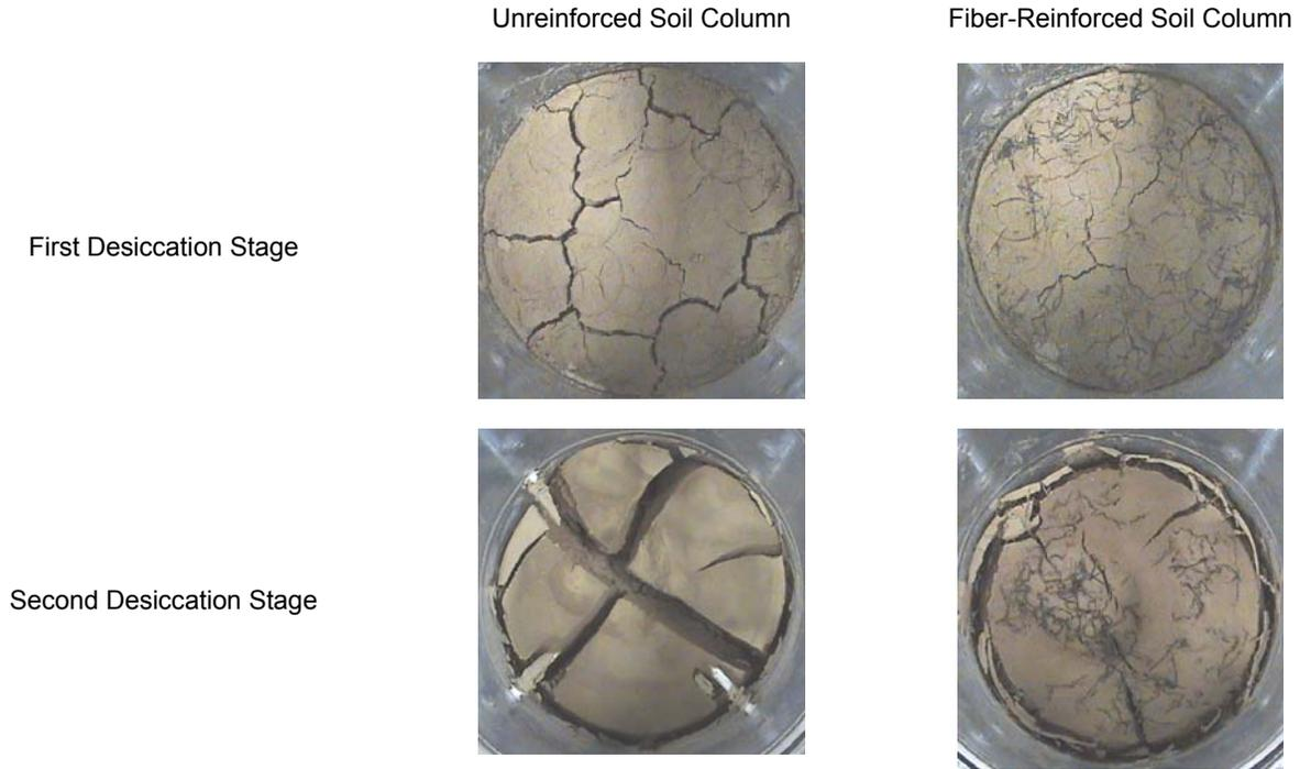
Figure 5. Examples of Soil Column Surface Pictures for the Soil Columns for Both Desiccation Stages (Photos Taken at 48 Hours).
