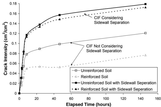
Figure 6. The Development of the Crack Intensity Factor With Time for the Soil Columns (First Desiccation Cycle).
