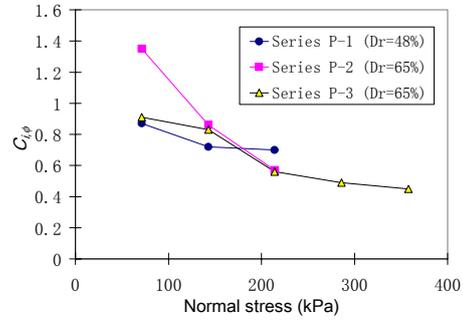
Figure 5. Coefficient of interaction as a function of normal stress
