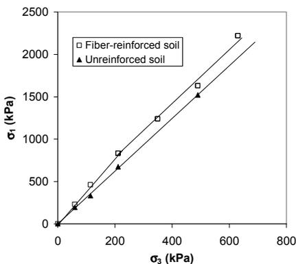
Figure 7. Shear strength envelope of fiber-reinforced soil tested under wide range of confining pressure (0.1% 100 mm long 360 Denier fibers)
