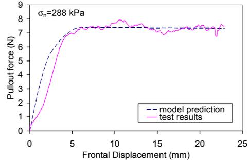
Figure 4. Fitting the pullout test result using the model
