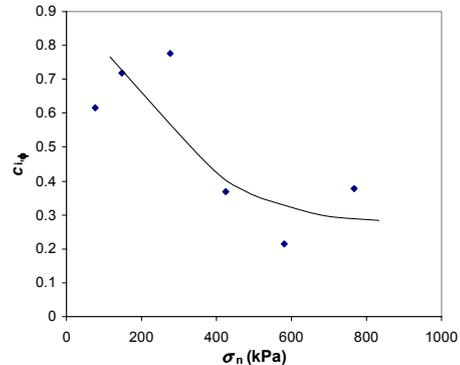
Figure 8. Coefficient of interaction back-calculated from triaxial test results
