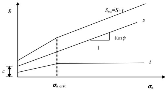
Figure 1. Representation of the equivalent shear strength according to the discrete approach
