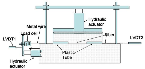
Figure 2. Setup of the fiber pullout test
