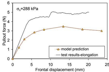
Figure 6. Comparison of model calculated fiber elongation and results from pullout test
