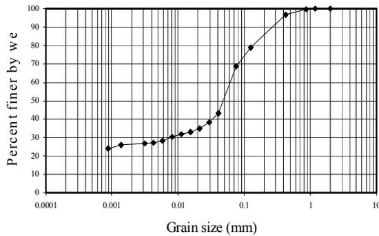
Figure 1 - Granulometric Curve of silty soil used in the testing program
