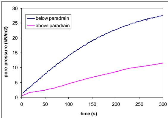
Figure 2 – Pore pressure during consolidation versus time
