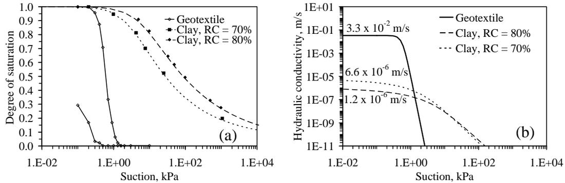
Figure 1: Hydraulic properties of compacted clay and nonwoven geotextile; (a) Water retention curves; (b) K-functions predicted from WCRs
