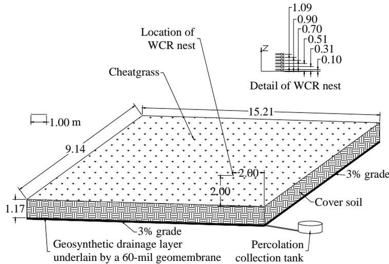
Figure 2: Schematic of the landfill test cover
