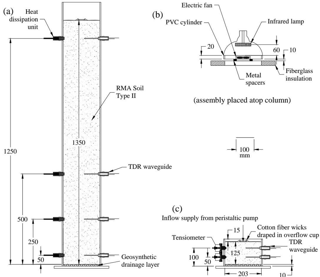
Figure 4: Column testing apparatus: (a) Profile A; (b) Evaporation setup; (c) Profile B
