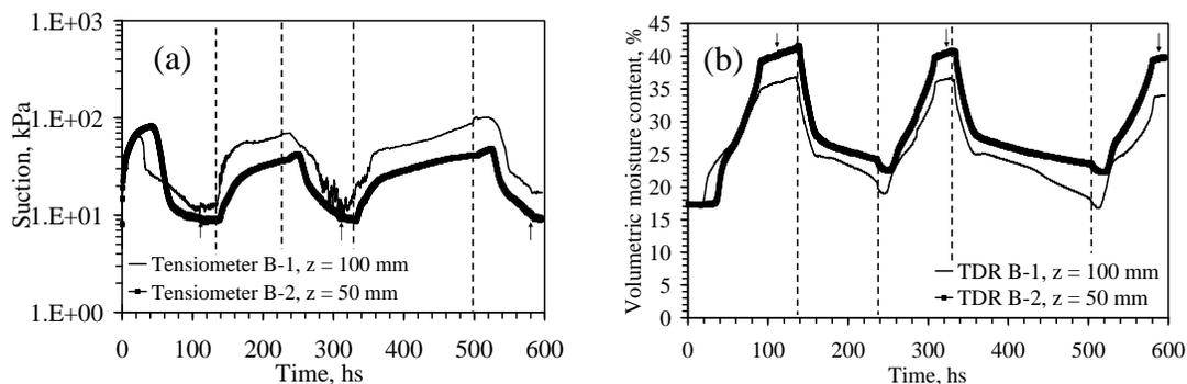
Figure 9: Profile B: (a) Suction; (b) Moisture content (Arrows denote breakthrough)
