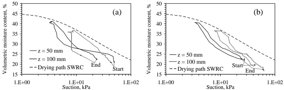
Figure 10: Transient WRC for Profile B: (a) Cycle 1; (b) Cycle 2
