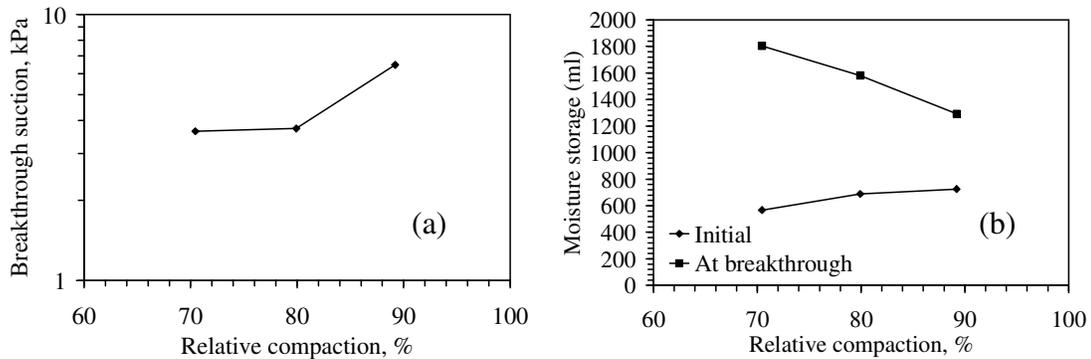
Figure 10: Effect of soil density: (a) Breakthrough suction; (b) Moisture storage
