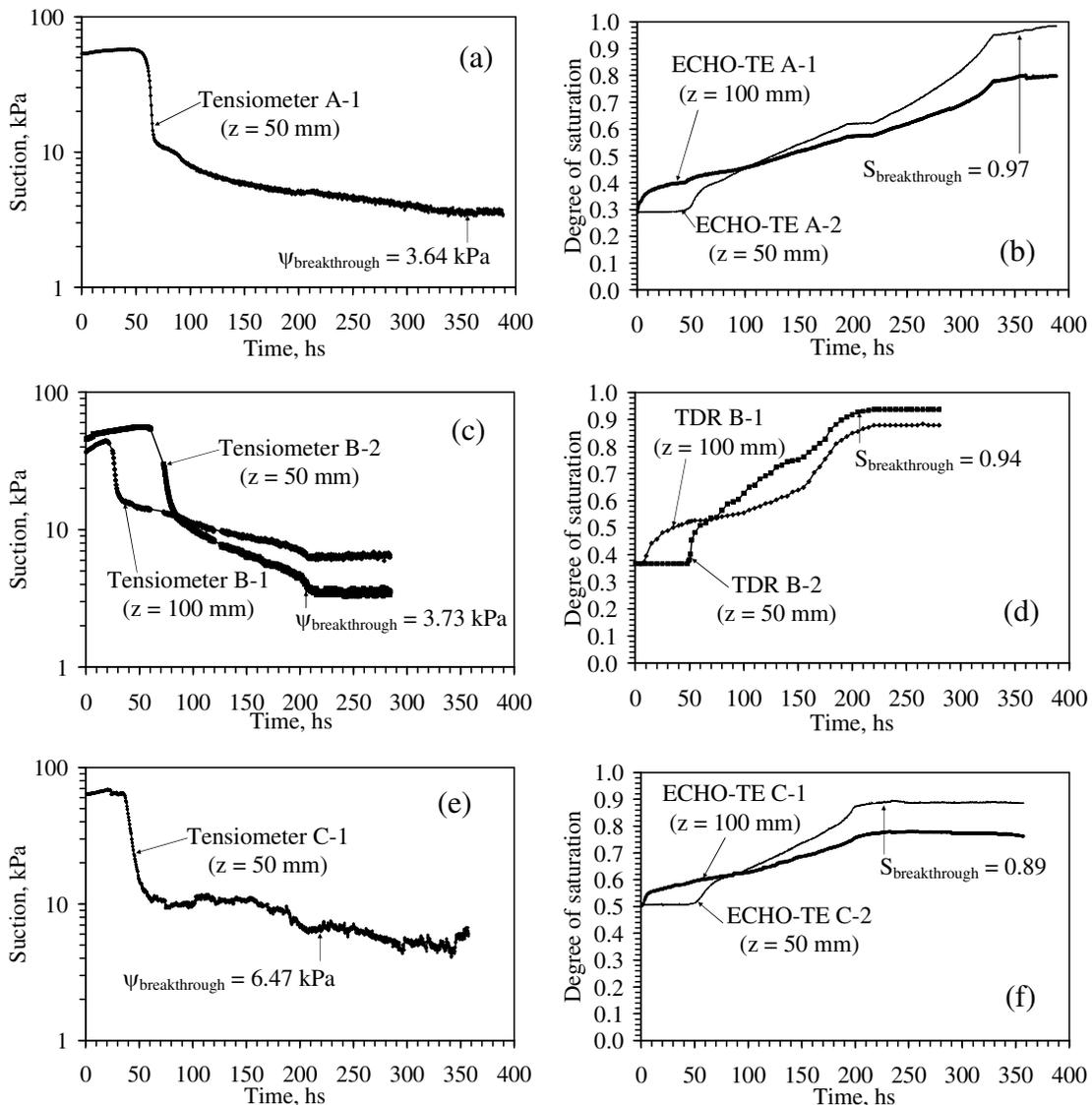
Figure 9: Profile A: (a) Suction; (b) Degree of saturation; Profile B: (c) Suction; Degree of saturation; Profile C: (a) Suction; (b) Degree of saturation
