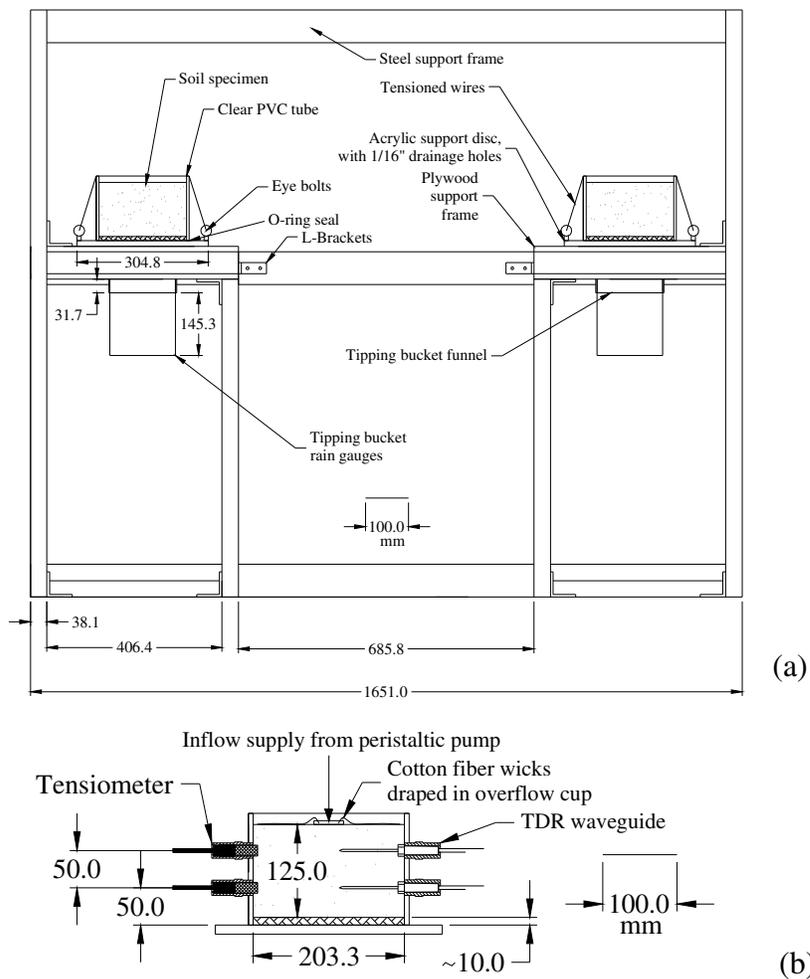
Figure 4: Column testing apparatus: (a) Support frame; (b) Column detail
