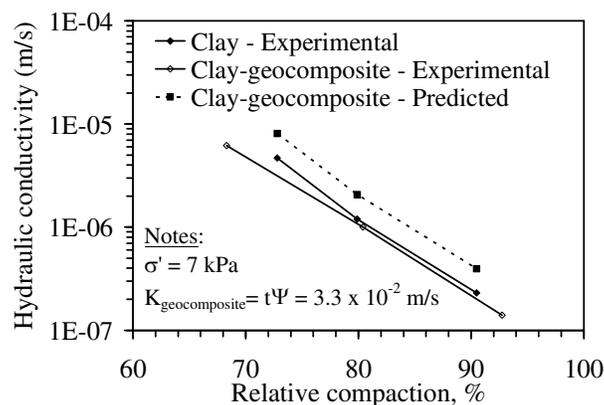
Figure 1: Hydraulic conductivity values of saturated specimens
