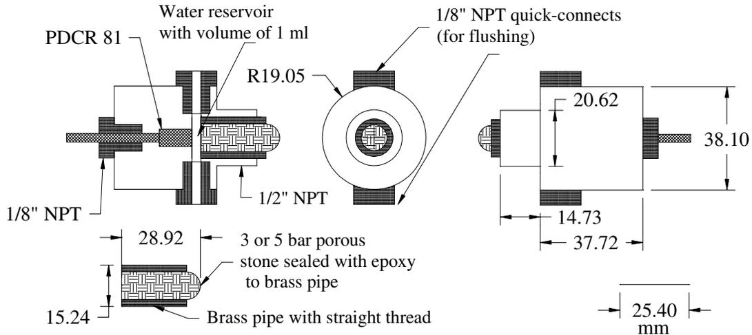
Figure 6: Schematic of the flushing tensiometer
