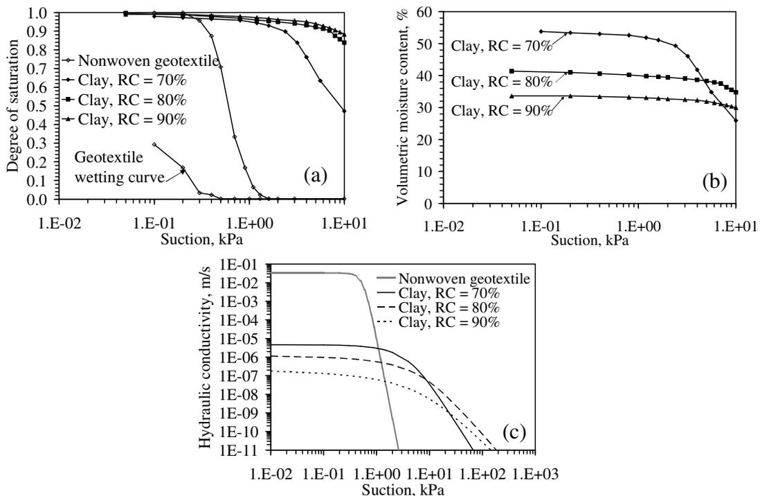
Figure 3: (a) WRC in saturation for geosynthetic drainage layer and clay; (b) WRC in moisture content for clay; (c) Predicted K-functions
