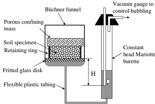
Figure 2: Hanging column apparatus
