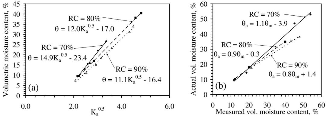
Figure 5: Calibration curves for the (a) TRASE and (b) ECH<sub>2</sub>O-TE systems
