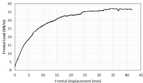
Figure 2. Frontal pullout load-displacement behavior
