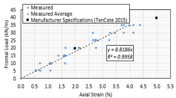
Figure 7. Reinforcement unconfined tensile behavior
