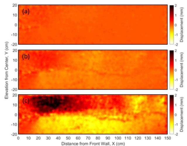
Six artificial gravel particles were stacked in a vertical array, centered in the box and located 30.5 cm ( $X = +30.5$  cm) from the front wall to measure the horizontal deformation. Soil
