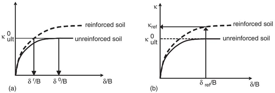
Figure 7. Reference parameters: (a)  $\delta^f/B$  definition; (b)  $\kappa_{ref}$  definition.
