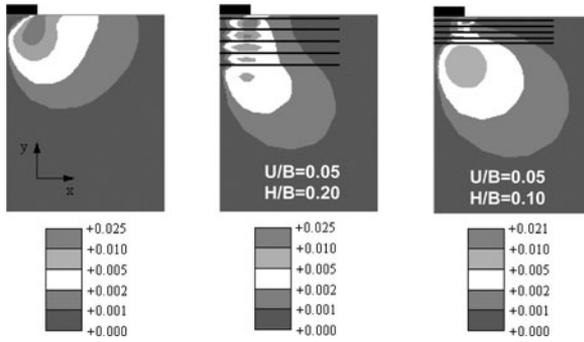
Figure 12. Horizontal displacement (m) – rigid foundation ( $\delta_{ref}/B = 0.1$ ).
