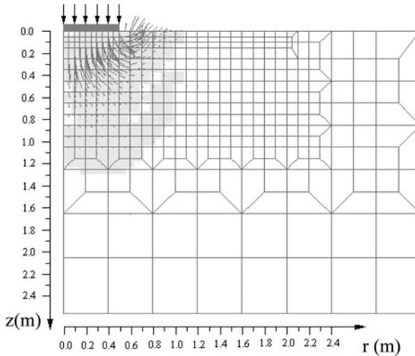
Figure 6. Failure mechanism – unreinforced soil.
