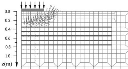
Figure 14. Influence of the first reinforcement layer depth – ( $\delta_{ref}/B = 0.1$ ).
