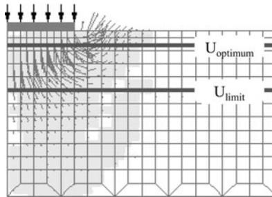
Figure 9. Optimum and limit reinforcement position.
