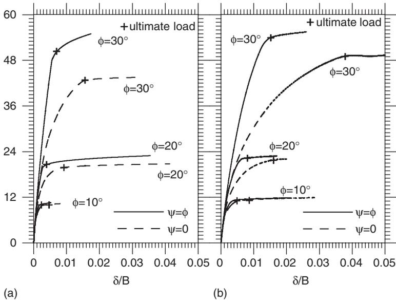
Figure 3. Load versus displacement curves: a) Flexible foundation; b) Rigid foundation.
