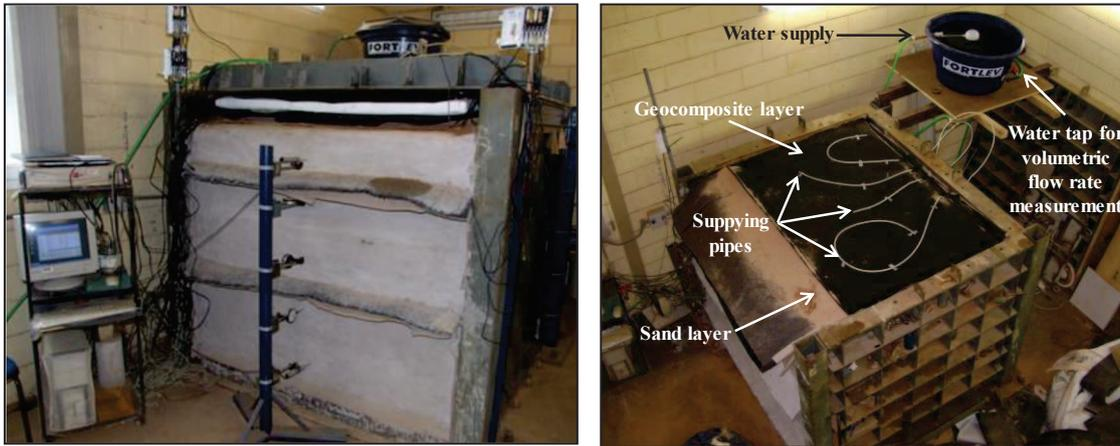
Figure 3. Full -scale reinforced wall model: (a) frontal view; (b) view of wetting system.
