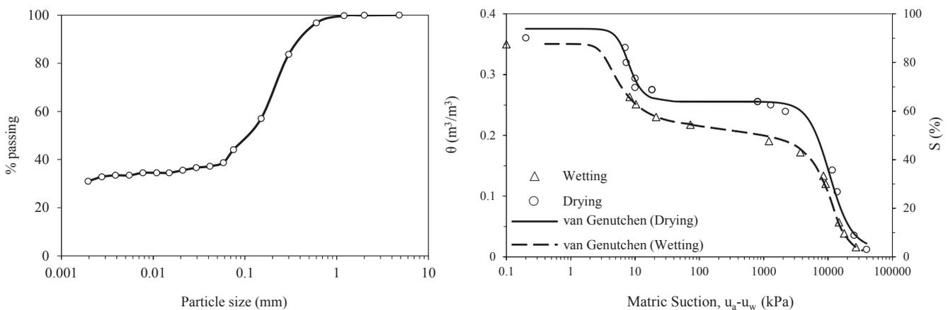
Figure 1. Properties of backfill soil: (a) Grain size distribution; (b) Soil water retention curve.
