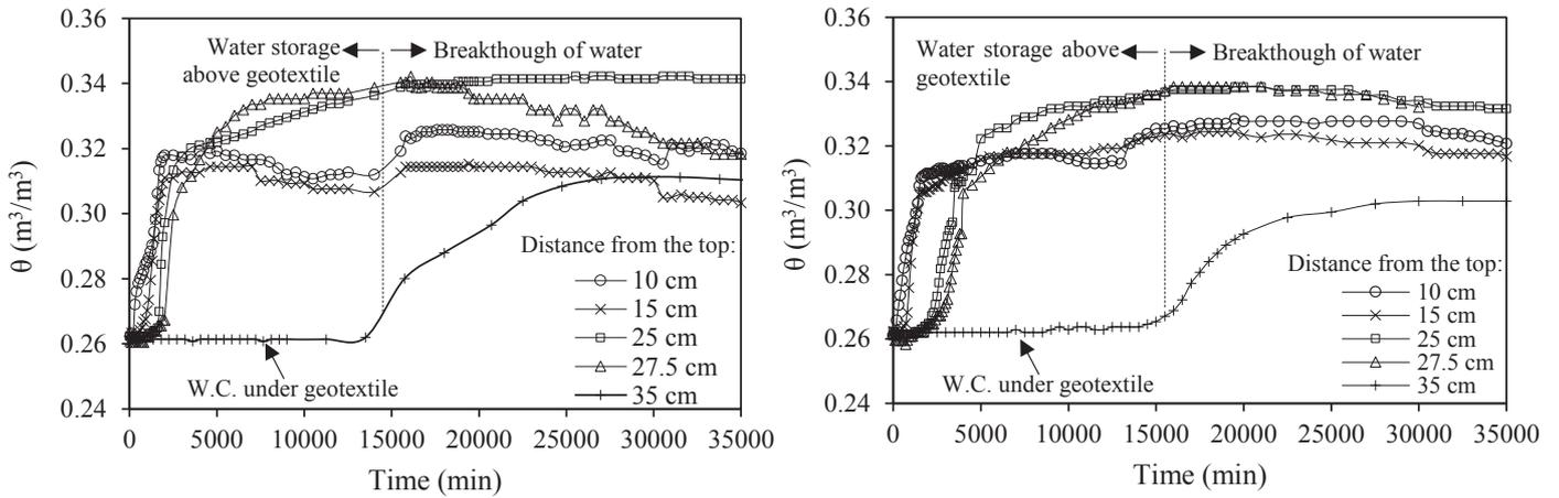
Figure 4. Time history of water content during infiltration: (a) in column location C1; (b) in column location C2.
