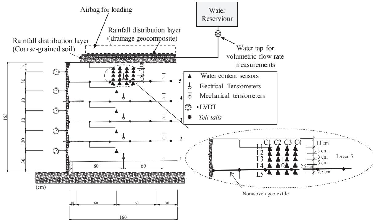
Figure 2. Cross section of the full-scale reinforced wall model, instrumentation layout and wetting system.
