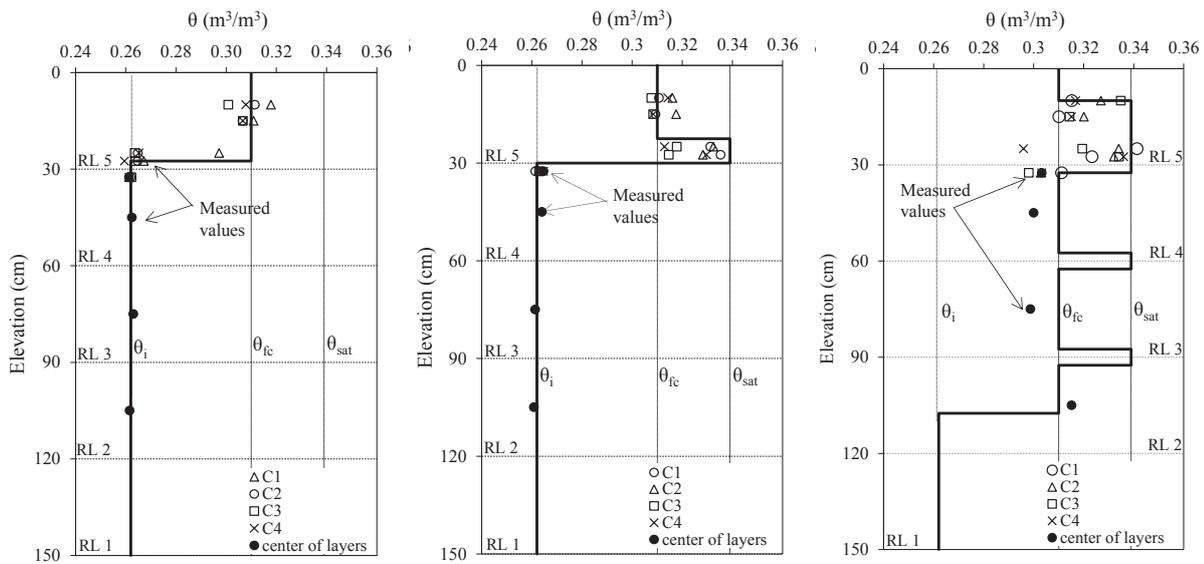
Figure 5. Infiltration profiles based on VWC after (a) 2000 min., (b) 10000 min. and (c) 30000 min. of irrigation.
