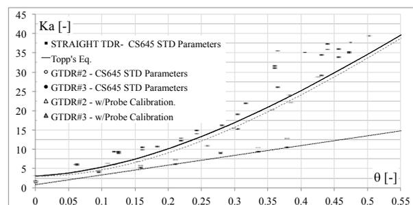
Figure 2. Three different calibration stages of GTDR
