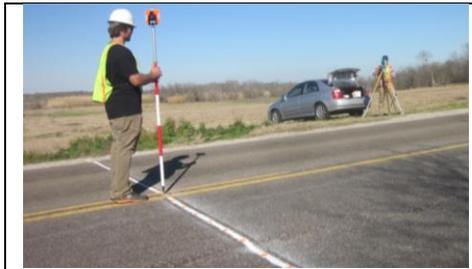
Fig. 4. Using total station and prism to monitor vertical deflection of the marked transverse sections
