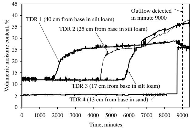
Figure 18. Volumetric water content with depth in Column 1 (McCartney *et al.* 2005)
