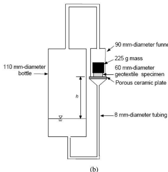
Figure 2. Hanging column test: (a) Conventional test used for soil specimens; (b) Modified test used for geotextile specimens (Stormont *et al.* 1997)
