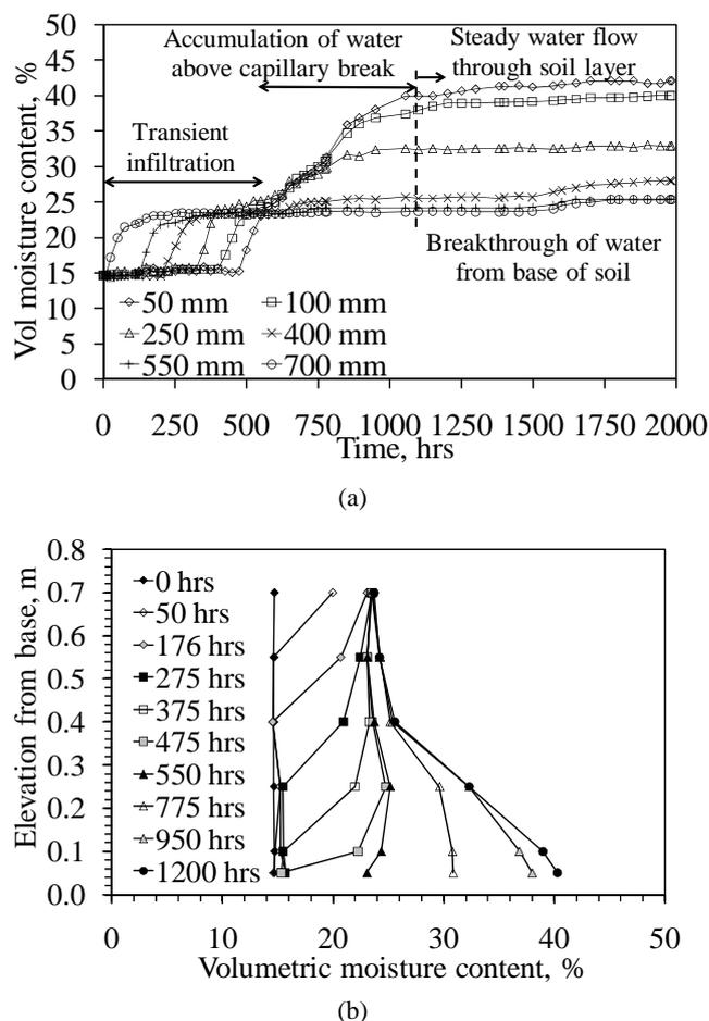
Figure 10. Results from column infiltration tests: (a) TDR water content time series for different heights from the base of a soil layer undergoing infiltration from the surface at a constant rate; (b) Water content profiles with depth for different times
