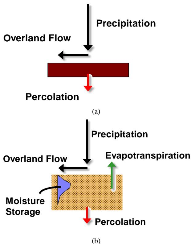
Figure 15. Components of the water balance in cover systems: (a) Resistive barrier; (b) Evapotranspirative cover
