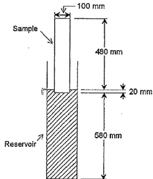
Figure 5. Test apparatus used to measure the in-plane water retention function of unsaturated geotextile specimens. (Lafleur *et al.*, 2000)
