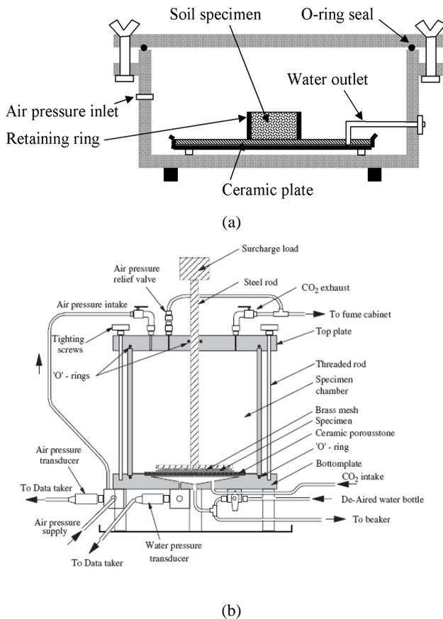
Figure 3. Pressure plate test: (a) Conventional test used for soil specimens; (b) Modified test used for geotextile specimens (Nahlawi *et al.* 2007a)
