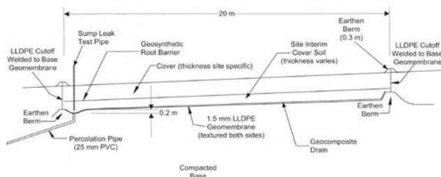
Figure 16. Schematic view of a typical pan lysimeter used for evaluation of the performance of alternative cover systems (Benson et al. 2001)
