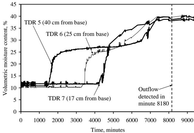
Figure 19. Volumetric water content with depth in Column 2 (McCartney *et al.* 2005)
