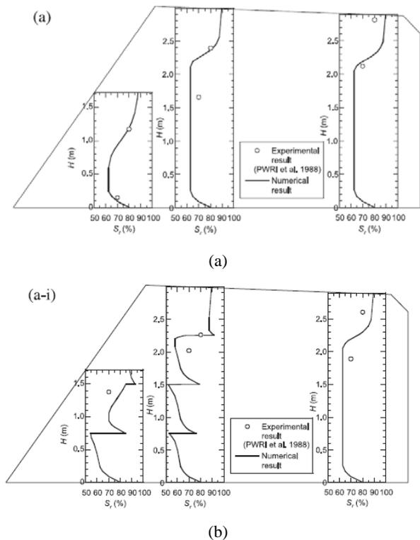
Figure 12. Comparison between water profiles in a retaining wall: (a) without reinforcements; (b) with geotextile reinforcements (Iryo and Rowe 2005b)
