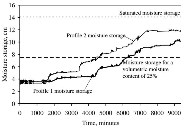
Figure 20. Water storage in Columns 1 and 2 during infiltration and at saturation (McCartney *et al.* 2005)
