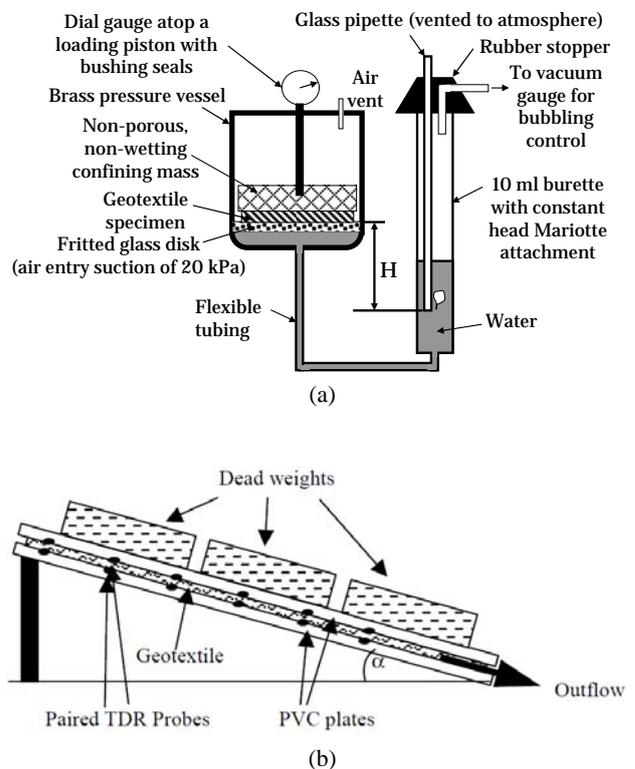
Figure 9. Equipment to measure the hydraulic conductivity of unsaturated geotextiles: (a) Hanging column with outflow measurement; (b) Inclined instantaneous profile test (Morris 2000)
