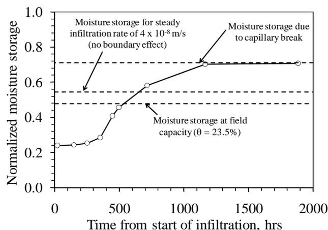
Figure 11. Increase in normalized water storage in the 300 mm of soil overlying the capillary break with time from the start of infiltration
