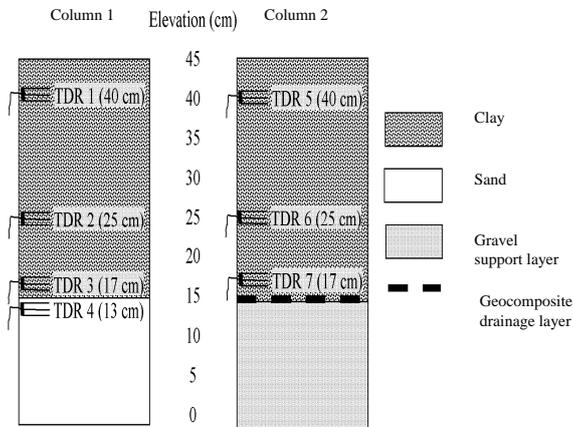
Figure 17. Schematic view of infiltration columns (McCartney *et al.* 2005)
