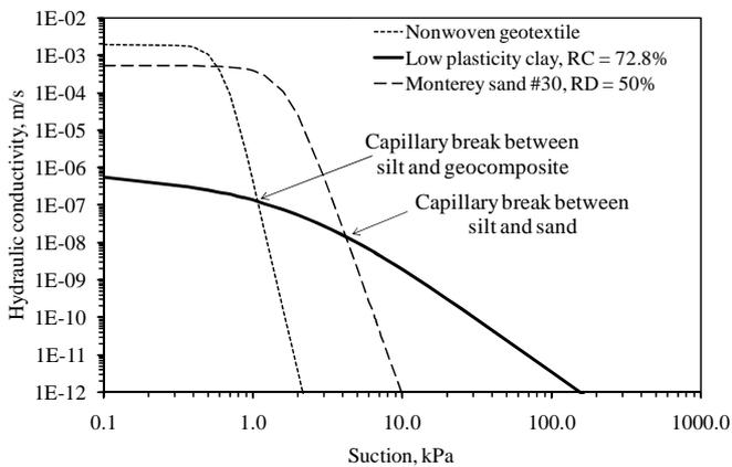
Figure 6. Typical  $K$ -functions for different geotechnical materials (after McCartney *et al.* 2005)
