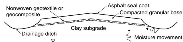
Figure 13. Nonwoven geotextile used as a hydraulic barrier in a flexible pavement
