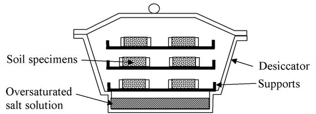
Figure 4. Conventional methods to determine the soil WRC using saturated salt solutions
