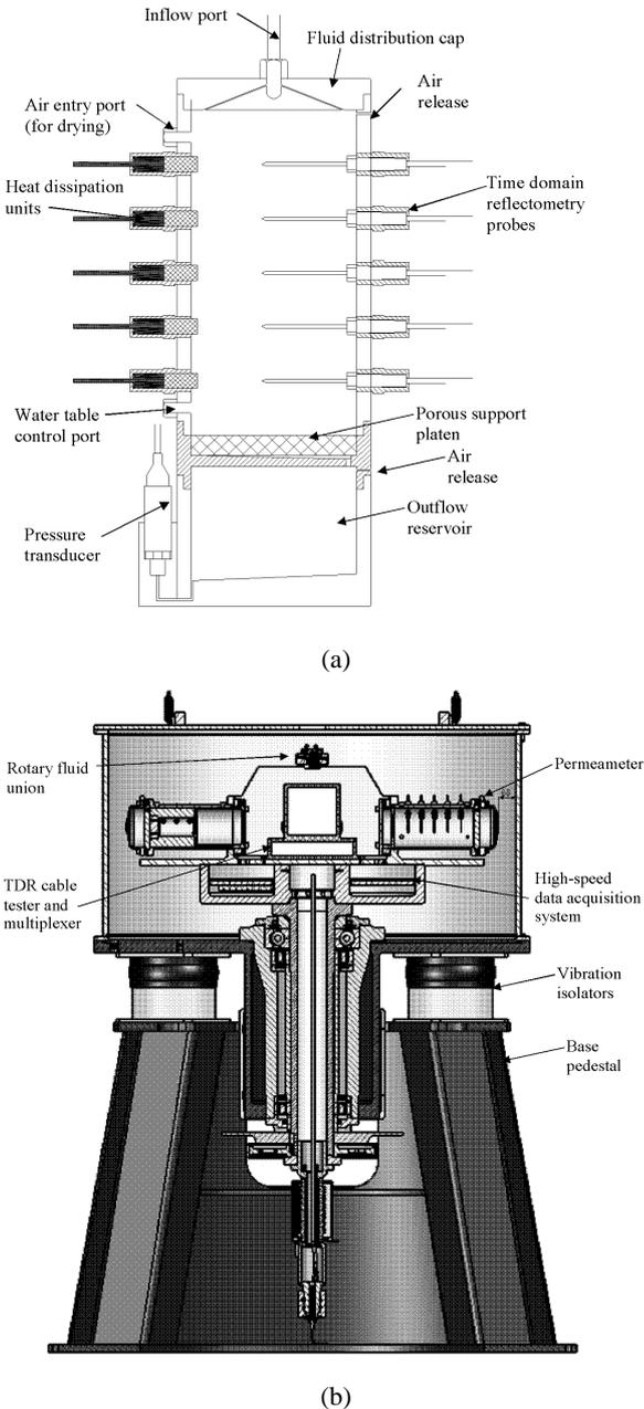
Figure 8. Permeameter for Unsaturated Soils: (a) Permeameter; (b) Centrifuge layout including a permeameter
