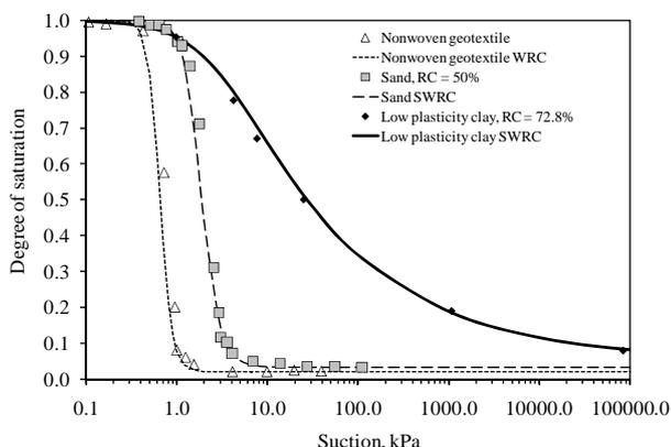
Figure 1. Typical WRCs for different geotechnical materials (after McCartney *et al.* 2005)
