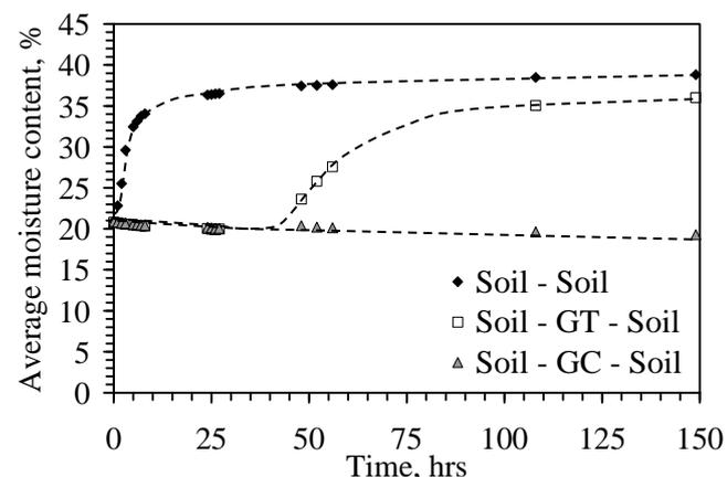
Figure 14. Water content changes due to capillary rise in different soil-geosynthetic systems (McCartney *et al.* 2008)
