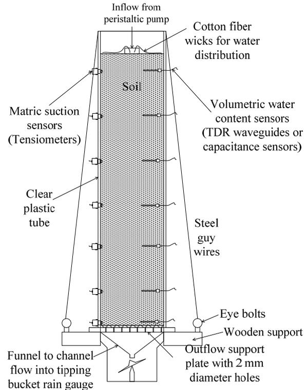
Figure 7. Column permeameter for unsaturated flow testing: (McCartney and Zornberg 2010)
