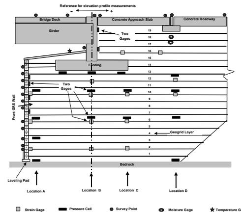
Figure 4. Instrumentation layout of section 800, showing location and type of instruments.
