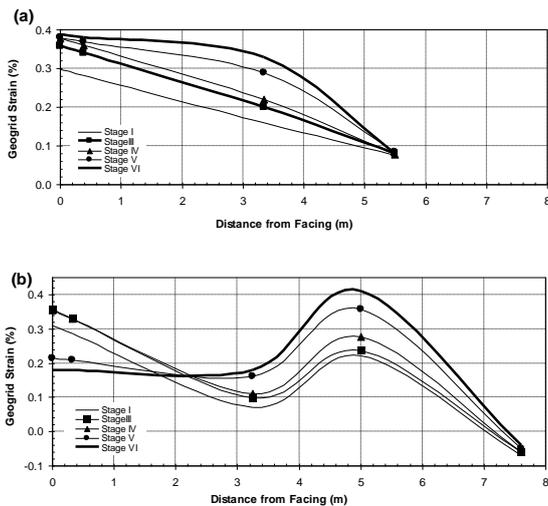
Figure 5. Geogrid strain distribution measured after construction stages along: a) geogrid layer 6, and b) geogrid layer 10.
