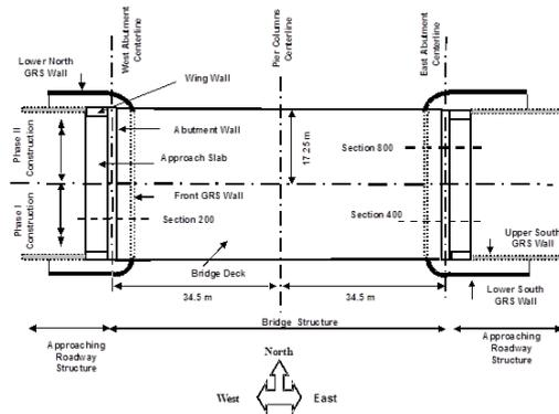
Figure 3. Plan view of the Founders/Meadows structure showing the locations of monitored sections (sections 200, 400, and 800).
