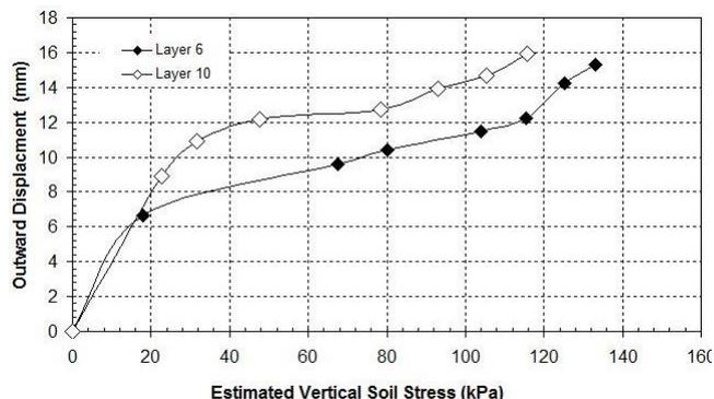
Figure 6. Outward displacements of the front GRS wall facing (section 800) at the elevation of geogrid layers 6 and 10, obtained from the strain gages results.
