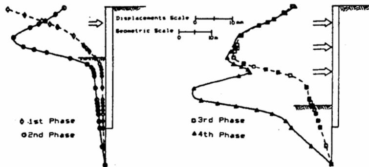
Fig.5. Wall displacements evolution during excavation
