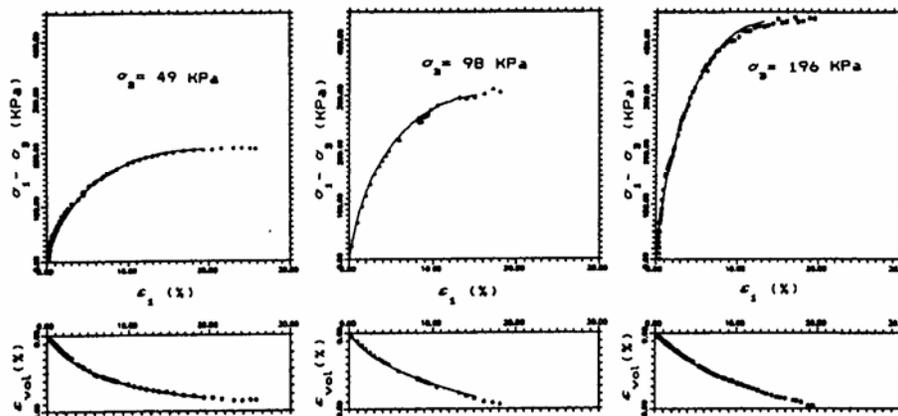
Fig.1 - Measured and Predicted "Red Clay" behavior in CTC tests
