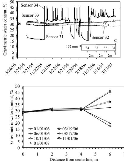
Figure 7: Horizontal moisture data from four sensors at Station 84 (a) Time series (b) Isochrones
