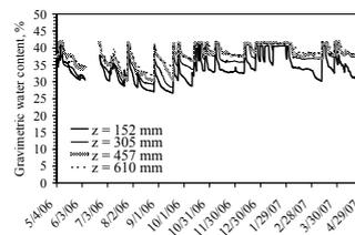
Figure 8: Times series for vertical moisture data from four sensors at Station 184
