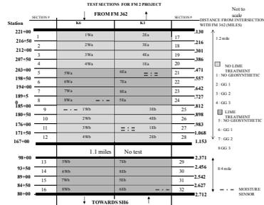
Figure 3: Layout of test sections at FM 2
