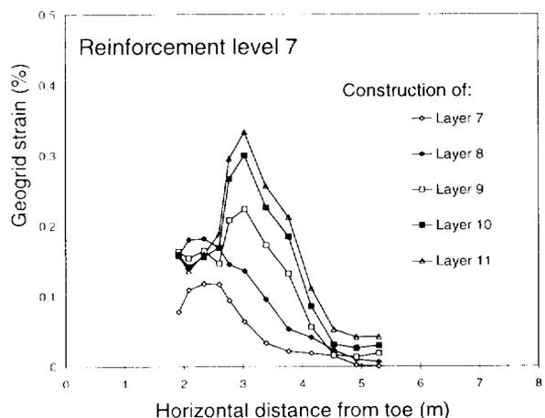
Figure 3. Estimated geogrid strains induced during construction.
