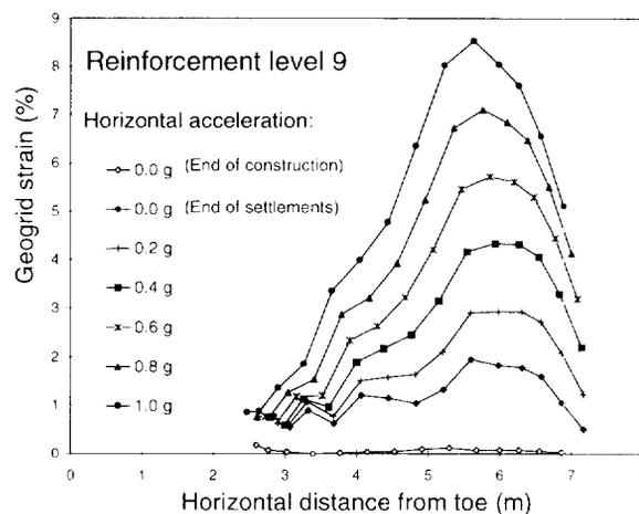
Figure 7. Estimated geogrid strains induced by seismic loads.
