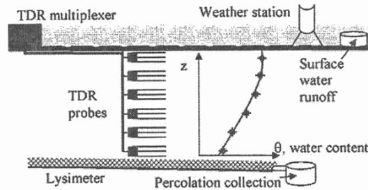
Figure 2. Monitoring system layout.
