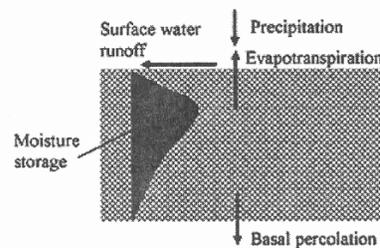
Figure 1. Schematic of an evapotranspirative cover.
