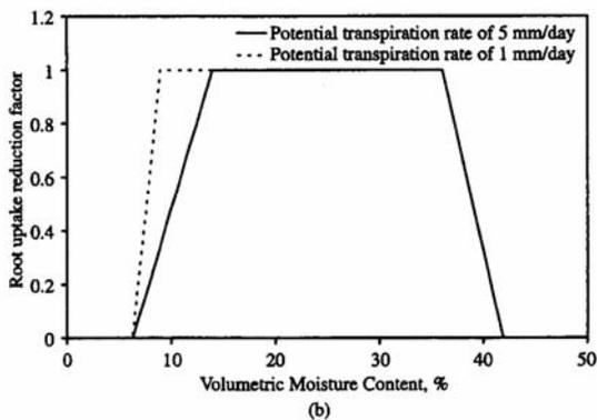
Figure 7. Root uptake information: (1) Root length distribution, (b) Root uptake reduction factor.
