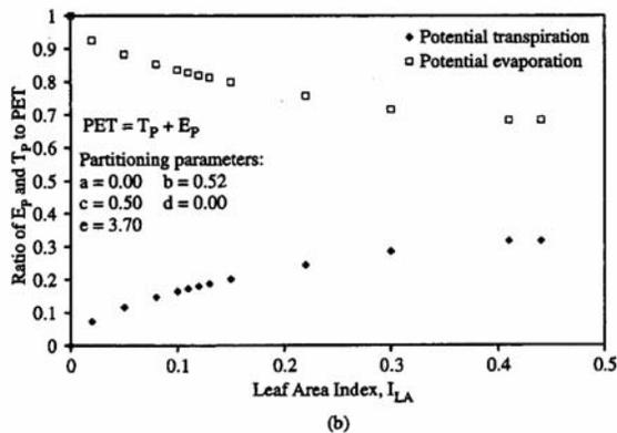
Figure 6. Agricultural data for partitioning PET into  $T_p$  and  $E_p$ : (a) Annual variation in leaf area index, (b) Ritchie model for partitioning  $E_p$  and  $T_p$  from PET.
