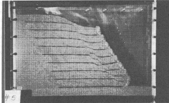
Figure 4. Failed geotextile-reinforced slope model
