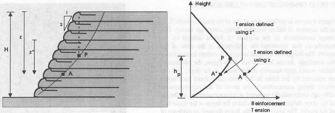
Figure 8. Reinforcement force distribution with depth for reinforced soil slopes
