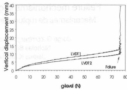
Figure 3. Settlements at the crest of a reinforced slope model
