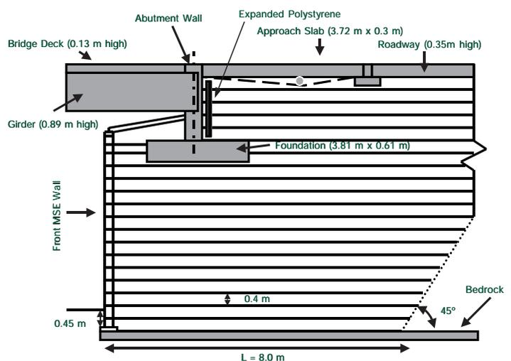
**Figure 2:** Typical monitored cross-section illustrating superstructure load transmitted through abutment walls.
