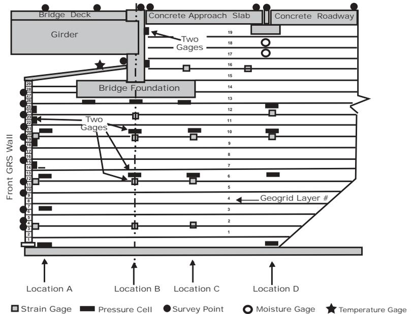
**Figure 3 :** Four critical locations (A,B,C,D) were instrumented in the phase II structure.
