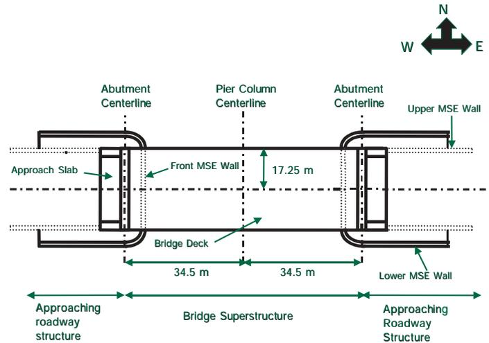
**Figure 1:** The new Founders/Meadows bridge structure, shown here in plan view, exhibits a wider span than the previous structure.
